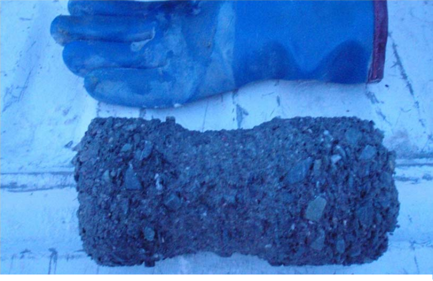
Photo 6: Drilled Core 11 (HB12-ND-CORE-DC11-QA-20120129), taken from ~ 1+25 on the upstream. Note that the central portion of the drill is narrower due to drill chatter (from dislodged gravel).
